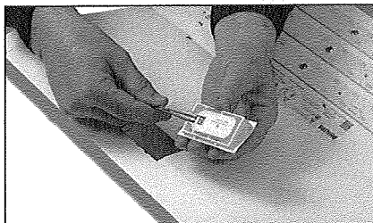
Step 4: Take these two wires and insert them into the sensor. They are not polarity sensitive.
